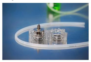
2. Hold the tubing with loading key, turn the key carefully and feed the tubing into the working position. Then fit the other end of the tubing into the other slot of housing. Do not twist the tubing.
