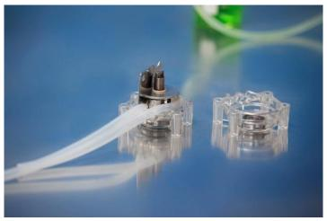
3. Remove the key, and put the housing back. Tighten the tubing properly by hand, then turn the rotor by key to move the tubing to the center position of the roller.
